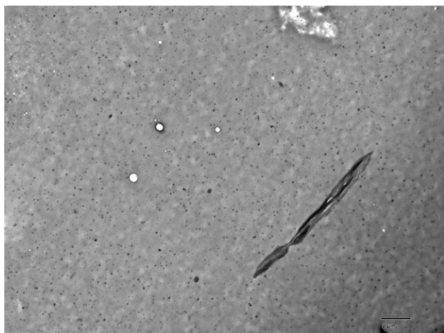
Figure 2. TEM micrograph of PLA-BCNC films containing 1 wt % BCNC. Scale markers correspond to 2 \mu\text{m} .
